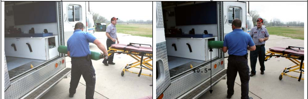
Positioning the O2 tank at waist level to slide it into the storage container in them ambulance located 40.5 inches above the ground.
