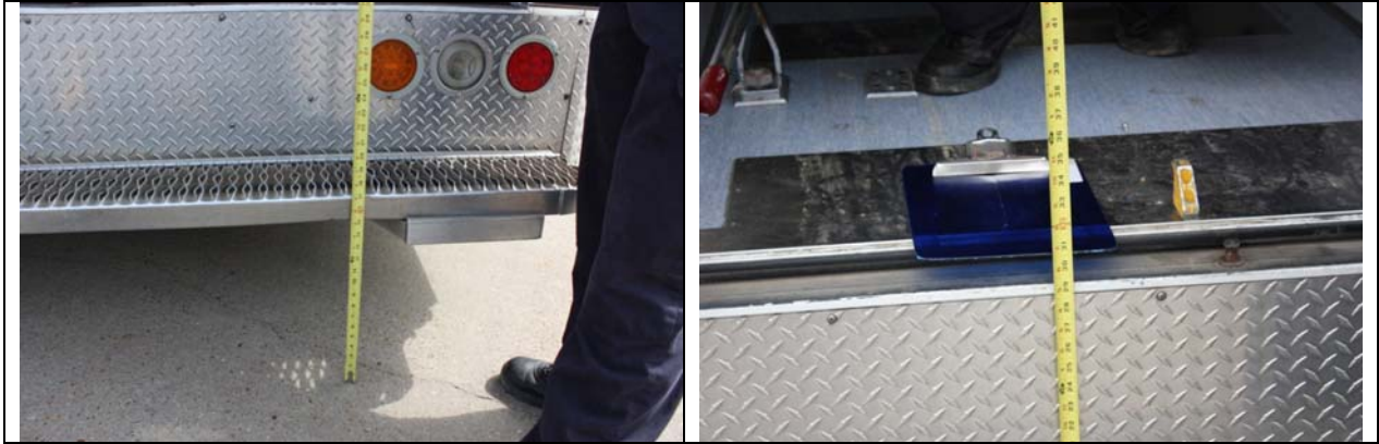
Climbing in and out of an ambulance requires ability to flex the hip and knee sufficiently to step up 17.5 inches for the 1 st step and 30.5” to the 2 nd step.
