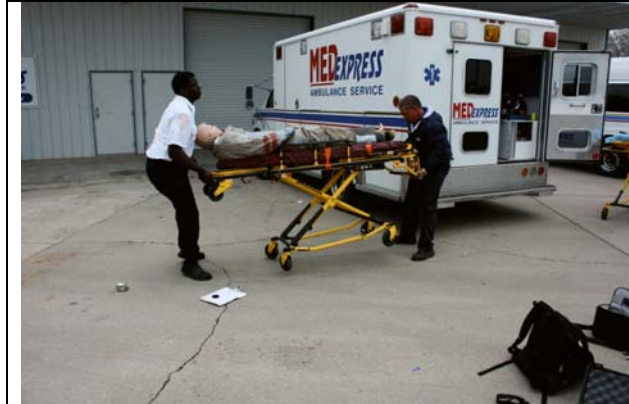
3. – 4. To fully elevate the stretcher, the hands are located 36.25” at the head end of the stretcher and 22” at the lowest of the two handles located at the foot end of the stretcher. Lifting a 200 lb person requires a lifting a weight of 170 lbs.
