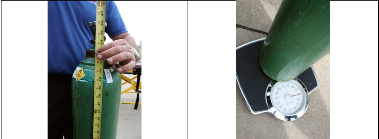
O2 bottles weigh 80 lbs and are 46 inches in height and 22.25 inches in outer diameter. They are moved on average 10 feet but can be carried by a dolly. Therefore, manual carrying of an 80 lb O2 bottle is not essential.
