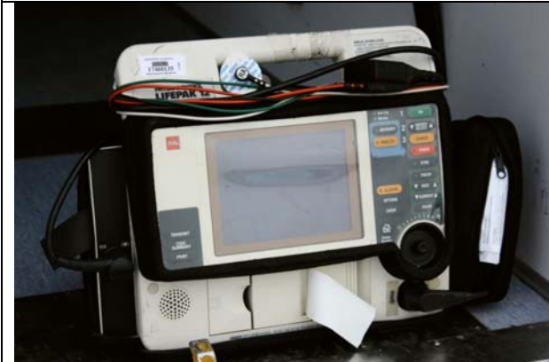
Lifepak Portable EKG Monitor measuring 19"x14" x 8.5" weighing 20 lbs is carried by a shoulder strap.
